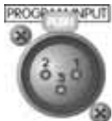
PROGRAM INPUT CONNECTOR XLR-3-31.
