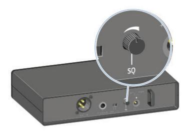
▶ Turn the control knob to the left or right to adjust the squelch.
