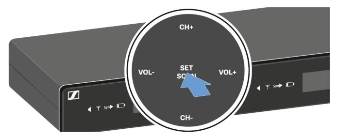
Press the CH+/CH- buttons to select a frequency bank (1 to 8).
