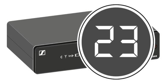
▶ Press the SET/SCAN button to accept the selected channel.
