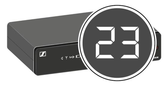
▶ Press the SET/SCAN button to accept the displayed channel.
