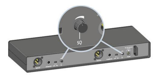
► Turn the control knob to the left or right to adjust the squelch.
