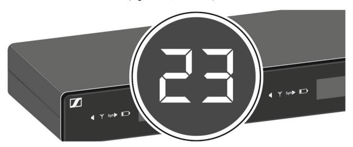
▶ Press the SET/SCAN button to accept the selected channel.
