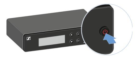
To switch the receiver to standby mode:
