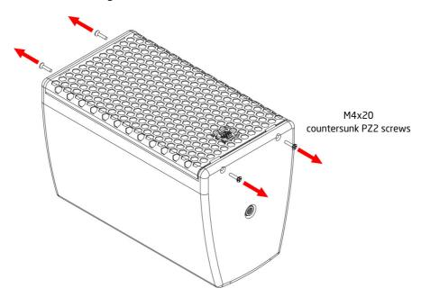
2. To replace the grille, position the grille on the front of the EMS-51X and ensure the threaded fittings on the grille are lined up with the mounting holes – gentle pressure may be required. Replace the four M4x20 countersunk screws and ensure they are both are started in their threads before beginning to tighten. Ensure they are all tightened evenly so that the grille sits straight and flat and does not rattle. Be careful not to over-tighten as this will distort the grille.
