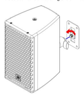
Once the WP-41 is secured to the wall or ceiling, then the BM-41 can be screwed on to the protruding M10 stud.
