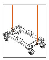
Use Admiral truss carriers Secure with sufficient lashing straps.
